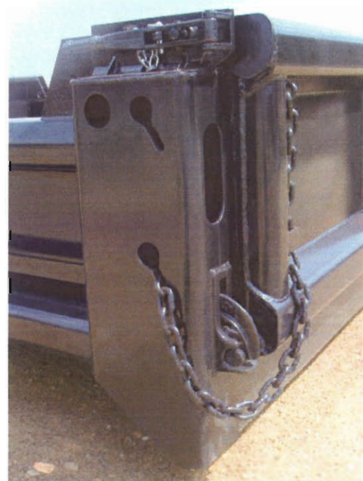
Pictured is a close view of the full-depth rear corner post with integrated chain adjusters and 9" deep 10 gauge high tensile steel rear bolster.
